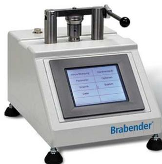
The **Viscograph®-E** measures the gelatinization properties of flour and native or modified starch, enzyme activity in flour (e.g. sprout), adjust the diastatic activity by adding enzymes (e.g. malt flour), influence of extrusion conditions onto the extruded product. Peak viscosity helps to predict flour quality to produce noodles with better texture characteristics.
