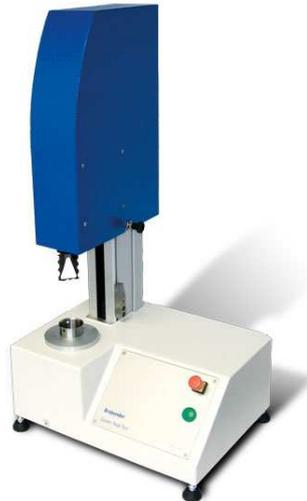
The **Glutograph®-E** instrument enables reliable, objective, and reproducible measurement of the stretching and elastic properties of washed wet gluten and dry gluten. The Glutograph® can test flour quality with regard to its suitability for noodle production, recognition of drying and heat damage of flour and dry gluten, and surveillance of the quality of dough during production.
