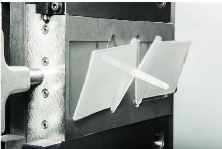
*The Brabender SpeciT Mold produces samples during the ongoing compounding process. For example, small plates in accordance with ISO 294-3 (2002), dumbbell specimens in accordance with DIN EN ISO 3167 or flow spirals.*
