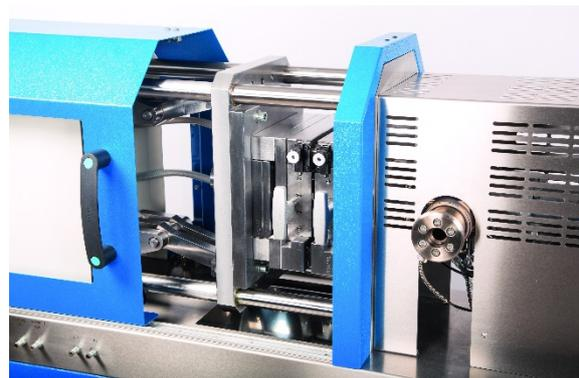
*The mould is opened and closed via a knee lever mechanism.*
